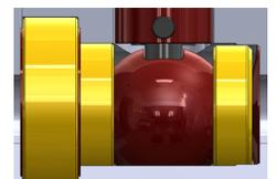
Trim set is vacuum tested to ensure a Class VI shut-off prior to rebuilding the valve
